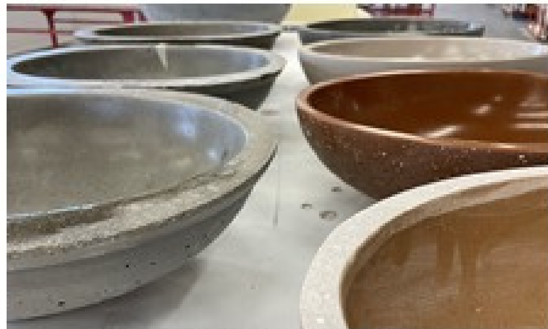
PRODUCTION OF CONCRETE WASHBASINS
